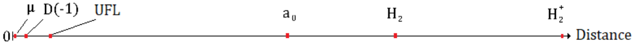
Fig. 6: Approximate relative distances between two nuclei where zero and a red dot represent the two nuclei positions for Muonic molecule \mu , ultra-dense deuterium D(-1) , Bohr radius a_0 (between proton and electron as red dot), hydrogen molecule H_2 and hydrogen molecule ion H_2^+ . Shown also is the upper fusion limit.
