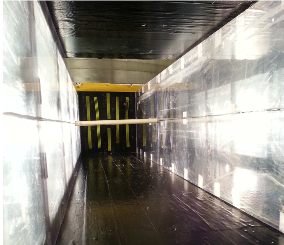
Figure B.26: Rig used for the vortex shedding tests, with a single circular cylinder inserted (Paper 3).
