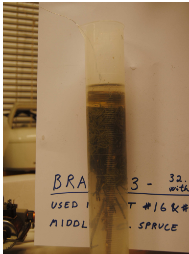
Figure B.20: Volume measurement of spruce branch 3 (Paper 4).
