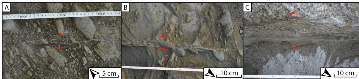
Figure 5.10: Stages of development; A) Low-displacement incipient bands ( D_{\max} < 5 cm) B) High-displacement mature bands/clusters ( 5 \text{ cm} < D_{\max} < 50 cm). C) Fully developed faults with a through-going principal slip surface ( D_{\max} > 0.5 m)
