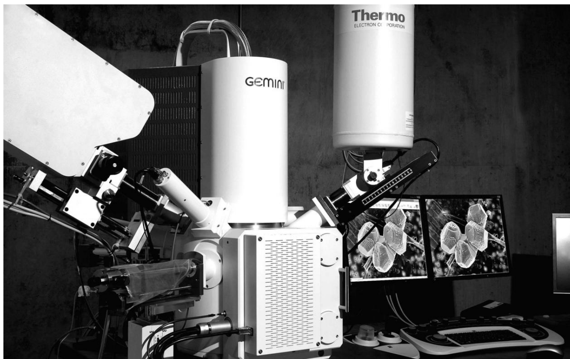
Figure 3.2: Supra 55VP Field Emission Scanning Electron Microscope used for thin section analysis. (Photo: Courtesy of Irene Heggstad, UiB)
