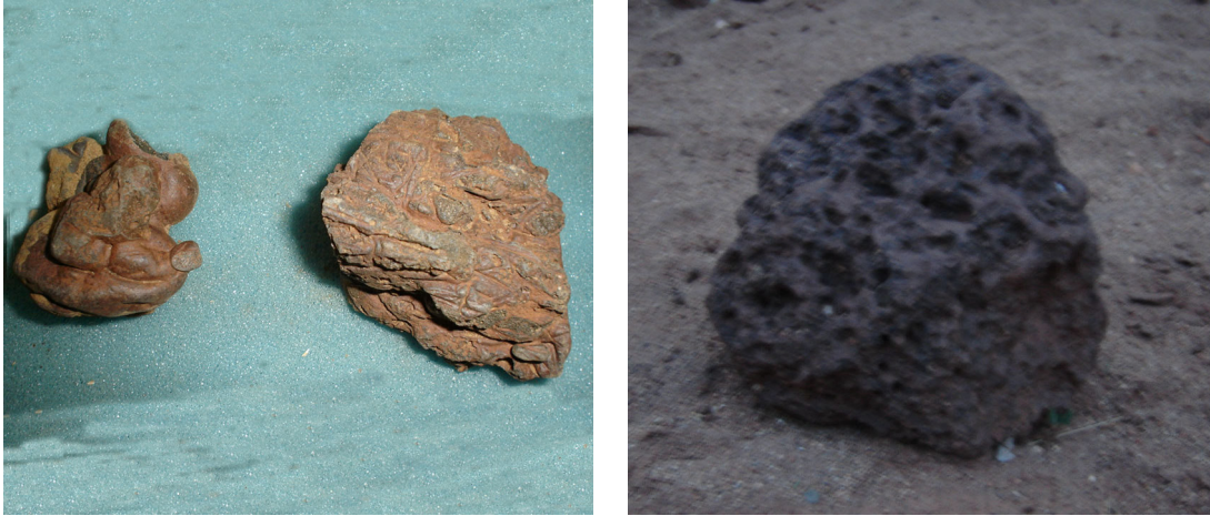
Figure 24 Some iron slag from Kangai Site (left) showing slag flow and (right) slag cake.
