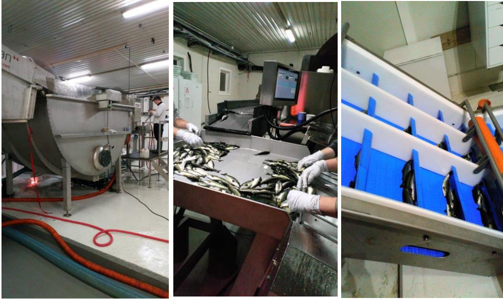
Figure 2.3: The left image shows the tank were the fish was sedated. This is a small tank, and not too many fish can be in this tank at the same time. This tank is closely monitored to keep oxygen and CO 2 levels acceptable. The middle image shows the table were the fish was sorted for size and arranged correctly. The right image shows the salmon after vaccination being transported back to a different 12m tank.
