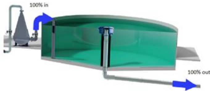
Figure 1.1: The basic principle of a flow-through system. Water flows through the facility and is discharged out of the facility. The water is not recirculated and there will be no need to treat the water at the outlet (Ole Gabriel Kverneland, Akva Group).
