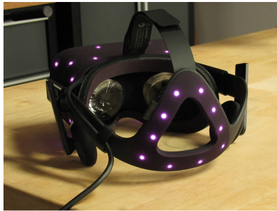
Figure 2.7: The Oculus Rift head-mounted display, with light emitting diodes showing, due to infrared sensitive camera imaging.[48]
