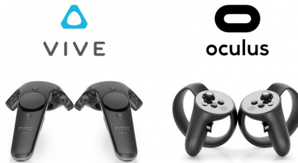
Figure 2.8: Positionally tracked hand controllers for the Oculus Rift(right), and HTC Vive (left).[49]
