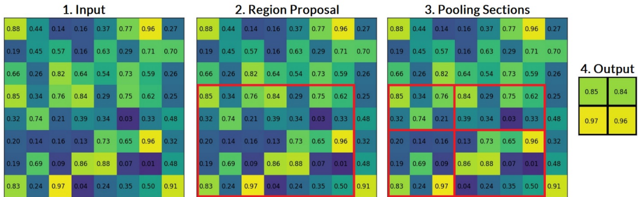
Figure 32: RoIPool step-by-step process – Adapted from [69]
