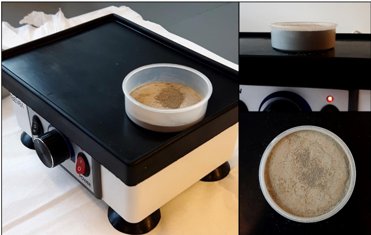
Figure 3.6: Packing sediment sample in polyethylene box. The instrument shook the sample gently, releasing air from the sediment.
