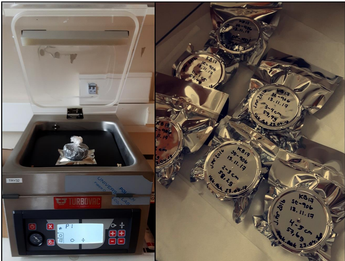
Figure 3.7: Left: a sample ready to be vacuum sealed using a Turbovac T20 Table Top Vacuum Packing Machine. A lead weight was put on top of the sample to prevent the sample from moving during the vacuum procedure, and to secure a result without air inside. Right: sediment samples after being sealed.
