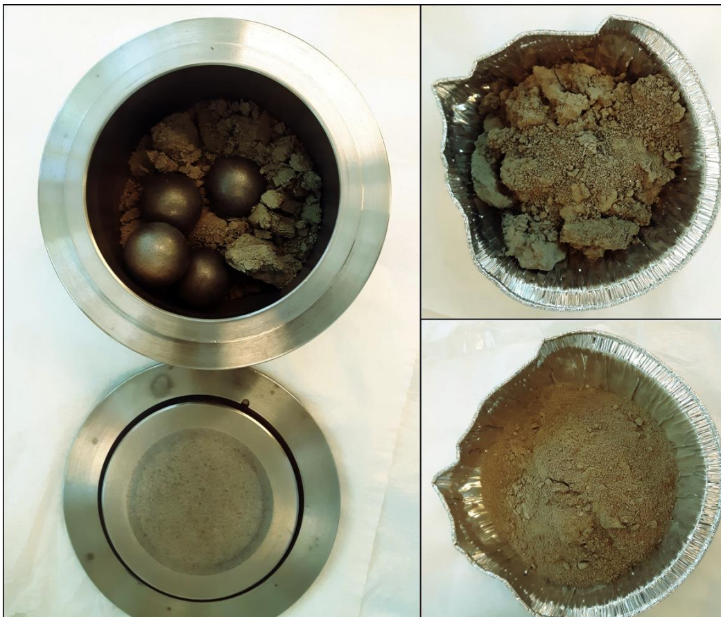
Figure 3.5: Left: A sediment sample ready to be homogenized using a ball mill. Right top: A freeze-dried sample before homogenizing. Right bottom: sediment sample after being homogenized.
