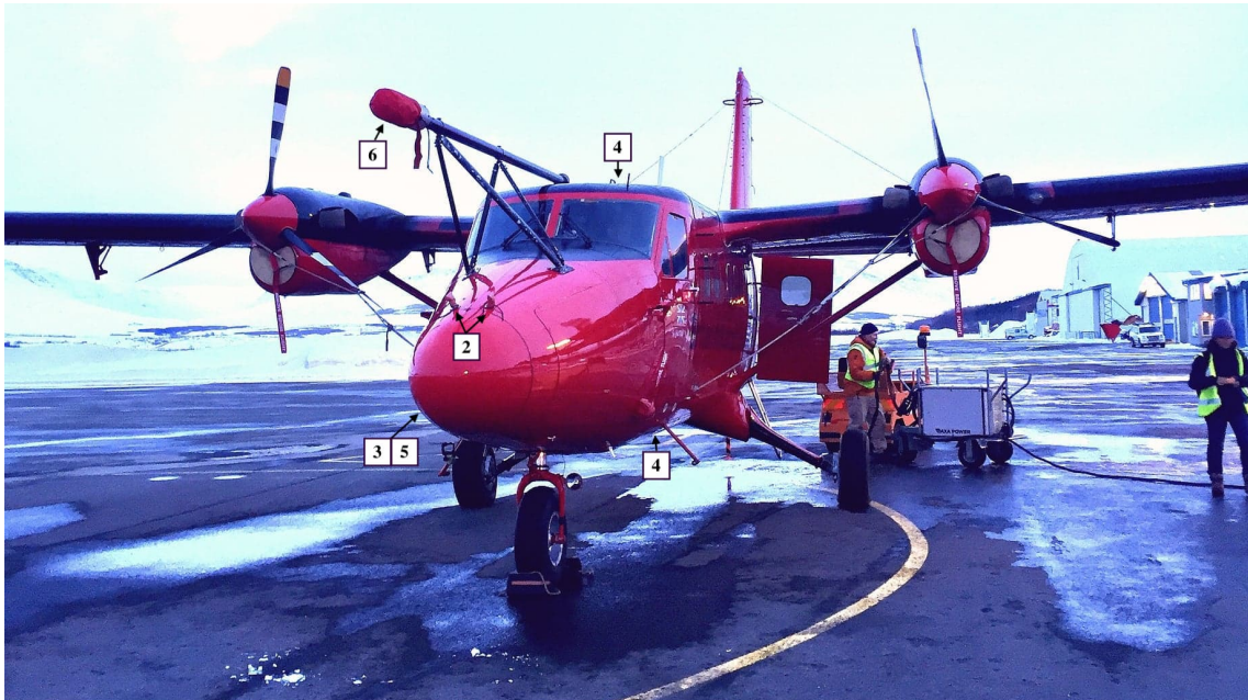
Figure 4.1: BAS Twin Otter Aircraft, equipped with MASIN instrumentation. The numbers refer to Table 4.1 to illustrate where the various instruments are located on the aircraft.
