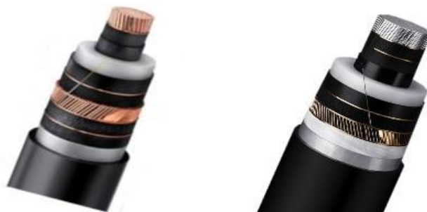
Figure 9.4 XLPE HVDC cables from Nexans (Cu & AL).
