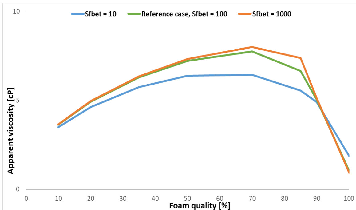
Figure 23: Foam apparent viscosity versus foam quality with varying Sfbet. The total injection rate is 240 mL/h. Foam reference case (Sfbet = 100, green curve), Sfbet = 10 (blue curve) and Sfbet = 1000 (orange curve).
