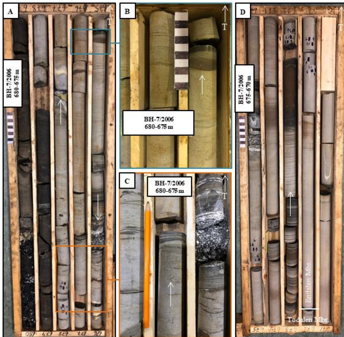
Figure 5.3: Sedimentary features of units 1 and 2 of the Firkanten Formation (core 7-2006). (A) Lower part of the Firkanten Formation (Totalen Mbr.). Abrupt change in lithology, from alternating mudstones and thin coal-layers to muddy sandstones (tidal channels). (B) Ripple-cross lamination in tidal channel. (C) Cluster of Macaronichnus trace fossils in tidal channel. (D) Rhythmites in the uppermost muddy sandstone (arrow).
