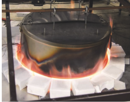
Figure 3. Fire testing with a propane mass flow rate of 0.6 g/s.
