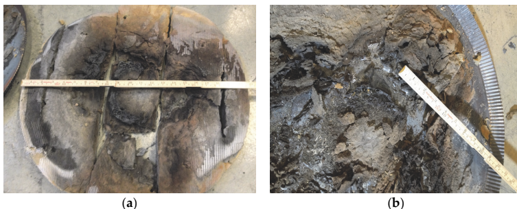
Figure 13. (a) Upper part of exposed thermal insulation after Test 2 and (b) lower part thermal insulation after Test 2.
