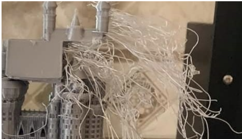
Figure 3.7: Printing on overhang without support results in spaghetti print
