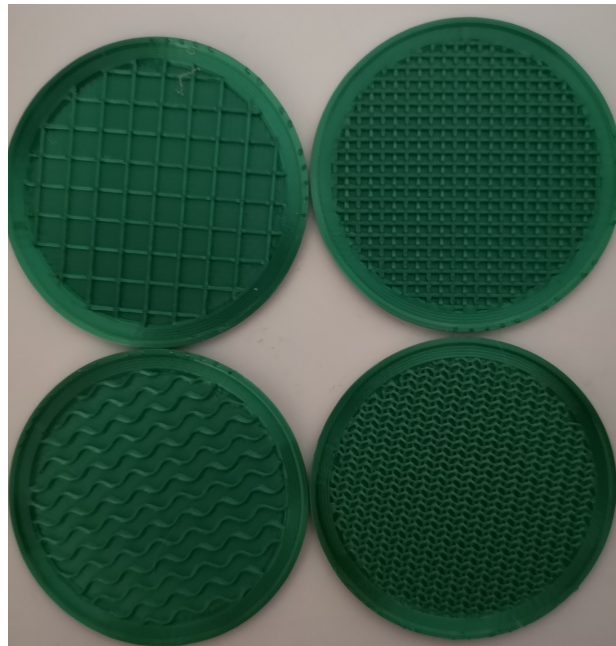
Figure 2.4: Same model printed using 4 different infill settings. The top-left and top-right objects are printed using grid infill pattern with 20% and 50% infill, respectively. The bottom-left and bottom-right have the same infill density as the top ones, but with a different infill pattern called gyroid .
