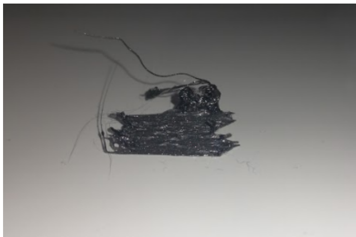
Figure 1.2: Print loosened from the print bed due to bad adhesion
