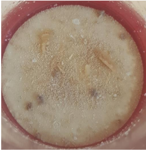
Figure 11: Undigested matter of salmon and possibly fish bones after the first filtration step
