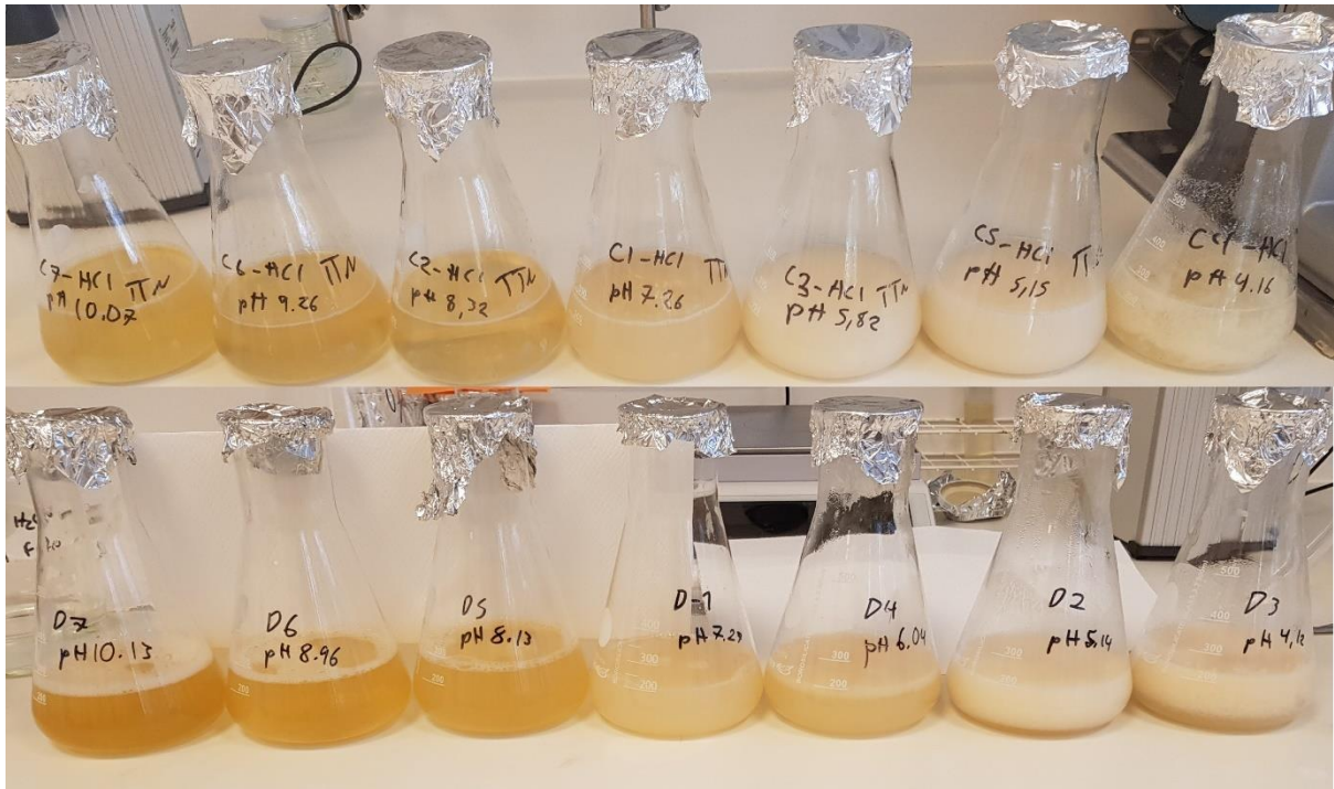
Figure 14: Erlenmeyer flasks sorted from basic to acidic (pH 10 → 4). Picture on top shows solutions titrated with HCl, while picture on bottom shows solutions titrated with citric acid.
