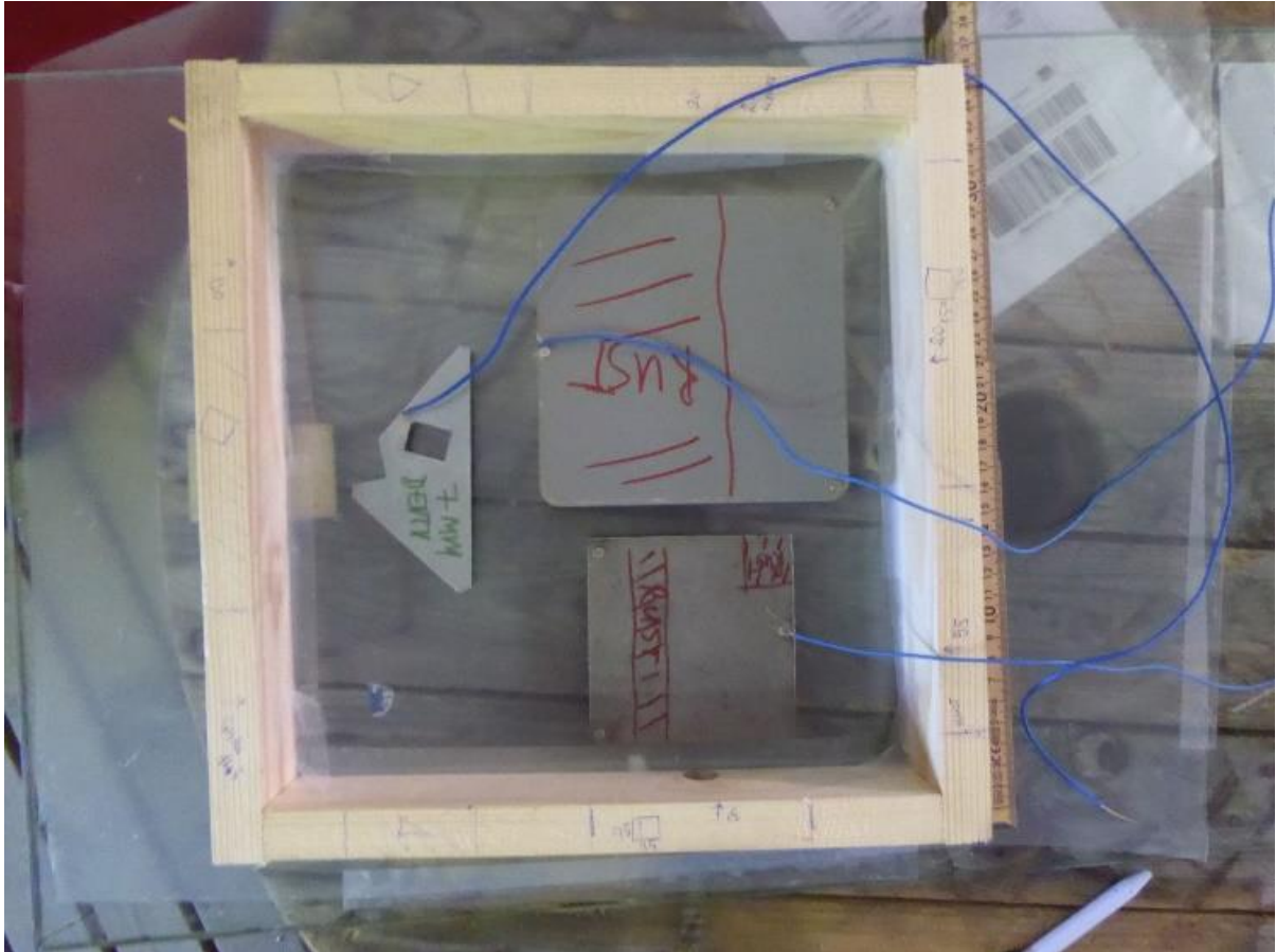
Figure 27: The contents of cement stone test sample 2 prior to casting, seen from the back of the sample. The areas marked "RUST" correspond to rust patterns on the opposite side of the plates.
