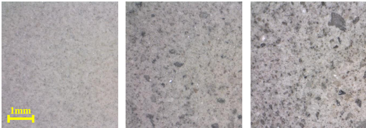
Figure 35: The surface of cement stone test sample 4 under a microscope. Three different areas are shown. Left: Smooth surface (untouched). Middle: Sanded surface. Right: The pattern above the corroded rebar.
