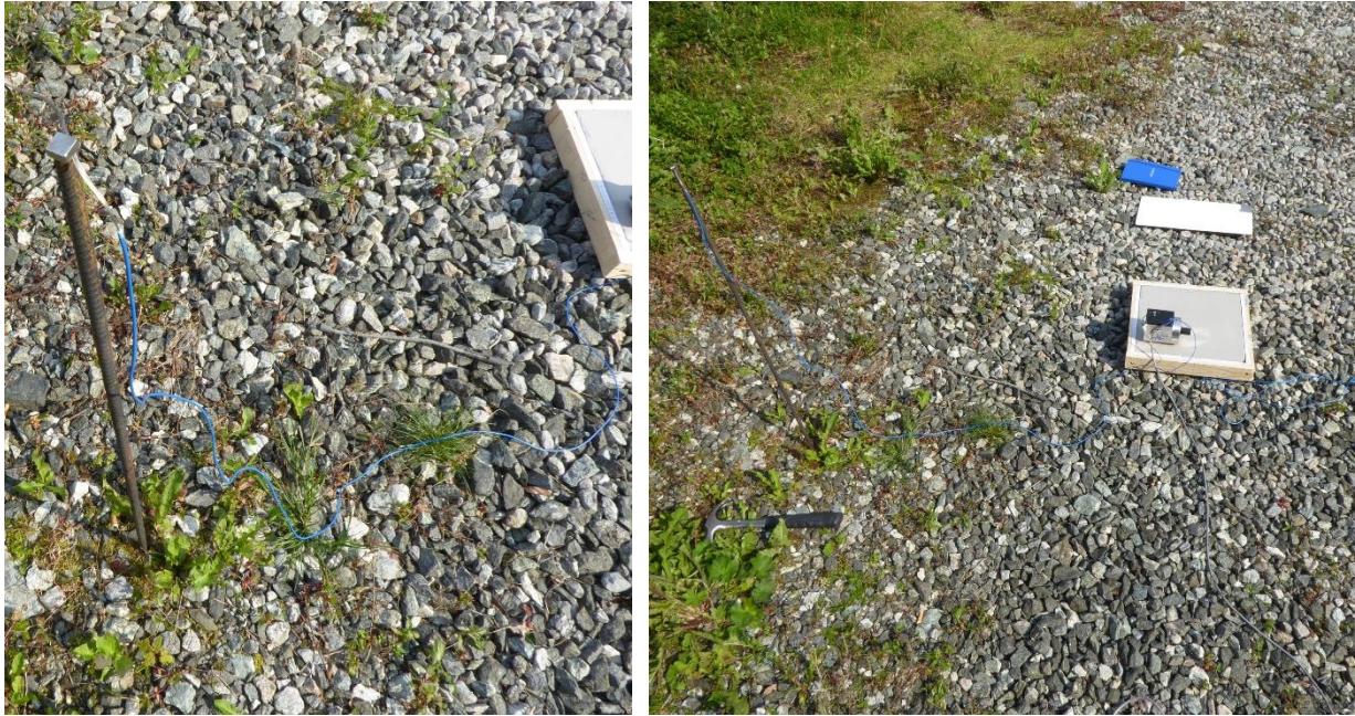
Figure 64: Field test outside NORCE, Fantoft. With the aim of testing measurements with a remote ground, a rebar was hammered into the ground and connected to the FKP. The FKP was then tested on cement stone test sample 3, which was connected to ground via a wire buried under the stones seen in the picture, producing a steady signal.
