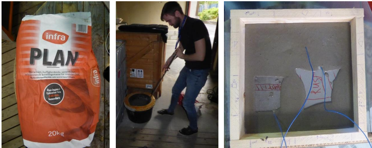
Figure 24: The cement used for all the cement test samples (Infra PLAN) is pictured on the left-hand side and the manual mixing of the cement with water is pictured in the middle. The right-hand picture is of cement test sample 2(ch.3.3.3) during casting. The back sides of the steel samples and the connecting wires are partly visible.
