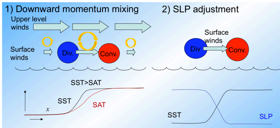
Fig. 4. Schematics of the (1) downward momentum mixing mechanism and (2) pressure adjustment mechanism. Courtesy of Shoshiro Minobe.
