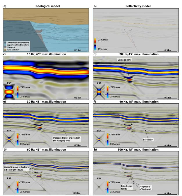
**Figure 5.7:** Synthetic seismic of Model 1 with different dominant frequencies on a range from 10 - 100 Hz of Ricker wavelets. The PSFs indicate the 2D seismic resolution of the seismic images. The color bar shows the relative color scale of amplitudes where the maximum values are absolute.
