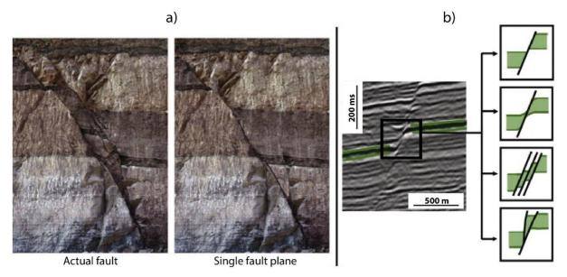
**Figure 3.3:** a) An outcrop example of a complex fault zone with several slip surfaces (left) and how it is often interpreted in seismic if the complexities of the core is not resolved (right). b) A plane structure of a fault in a 2D seismic section (left) and four different interpretations of the case (right). Modified after Botter et al. (2014).
