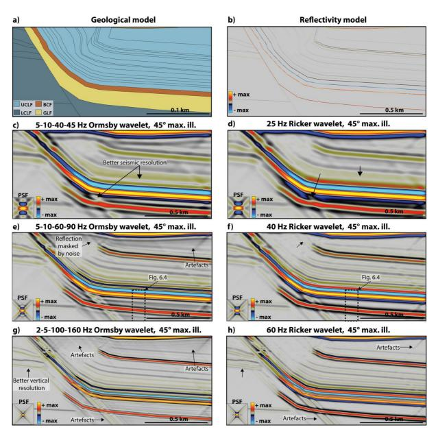
**Figure 5.16:** A comparison of the resulting synthetic seismic sections modeled with Ormsby wavelets of c) 5-10-40-45 Hz, e) 5-10-60-90 Hz and g) 2-5-100-160 Hz, and the corresponding dominant frequencies of the Ricker wavelet of d) 25 Hz, f) 40 Hz and 60 Hz. The black arrows point to features in the seismic that differs between the two wavelets.
