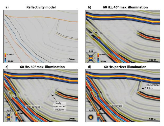
**Figure 5.12:** Synthetic seismic of a zoomed-in part of Model 4 (Fig. 5.6), where the maximum illumination angle is varied from 45°, via 60° to 90° (perfect illumination). The PSF is indicating the 2D seismic resolution and diplimited illumination. A Ricker wavelet of 60 Hz and vertical incidence are applied in all cases.
