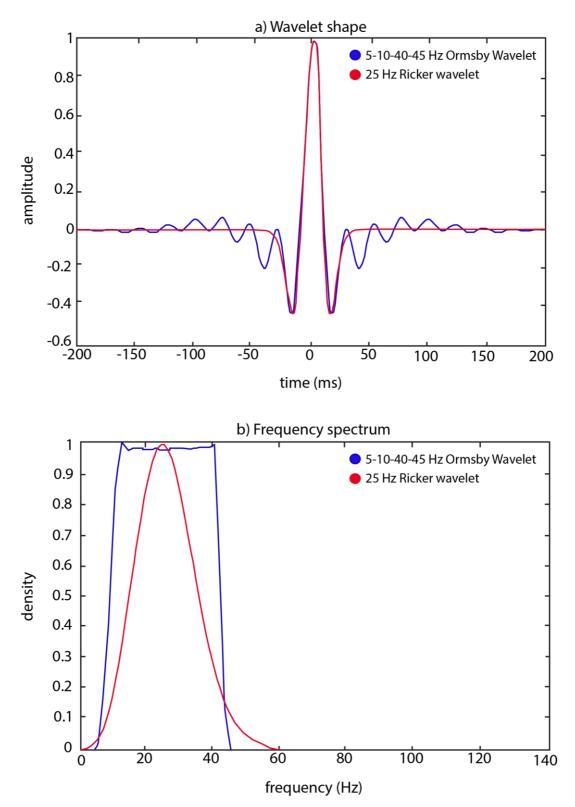
**Figure 5.15:** The (a) wavelet shape and (b) corresponding frequency spectrum of a 25 Hz Ricker wavelet and a 5-10-40-45 Hz Ormsby wavelet. Modified after Ryan (1994).
