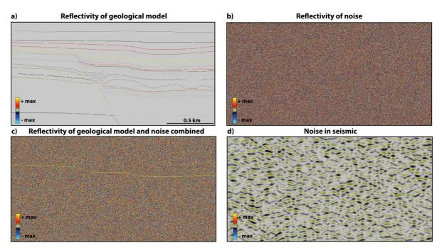
**Figure 5.9:** Reflectivity models of a) Model 1 and b) colored random noise. c) The reflectivity models in a) and b) combined. d) The seismic image of the input noise, corresponding to the reflectivity in b).
