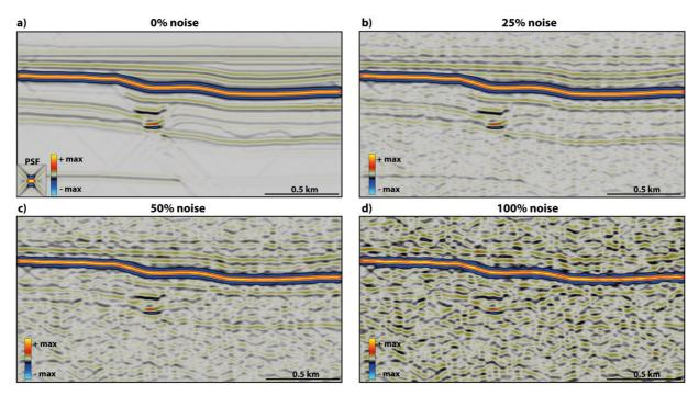
**Figure 5.10**: Synthetic seismic images of Model 1 where the level of random noise is systematically increased (0%, 25%, 50% and 100%). The geological model is presented in Fig. 5.6, and the reflectivity of Model 1 and the input noise, as well as the seismic of 100% noise, is presented in Fig. 5.9.
