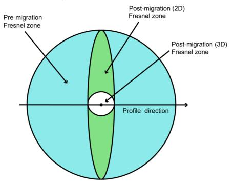
**Figure 3.4:** Seismic migration collapses the Fresnel zone in one dimension to an elliptical form for 2D seismic and reduces it to a small circle for 3D seismic. Modified after Simm and Bacon (2014).
