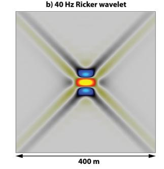
**Figure 5.17:** PSF of a) the 5-10-60-90 Hz Ormsby wavelet, and b) the corresponding Ricker wavelet of 40 Hz. Notice the difference in seismic artefacts between the two PSFs. The Ormsby wavelet generates a cross-pattern and circular artefacts, whereas the Ricker wavelet only generates a cross-pattern from the dip-limited illumination (here  $45^{\circ}$ ).
