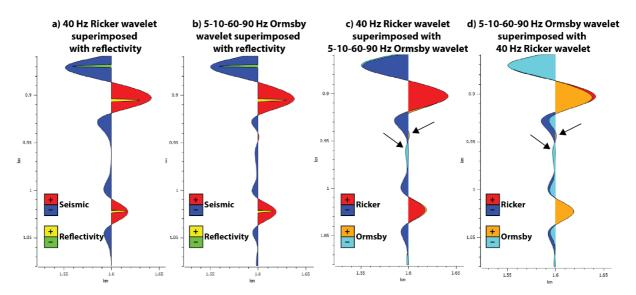
**Figure 6.4:** Superposition of wiggle traces from the seismic section of Model 4 (Figs. 5.16e and f). The first two plots show the reflectivity superimposed with the corresponding seismic wiggle trace generated with a) a 40 Hz Ricker wavelet and b) a 5-10-40-45 Hz Ormsby wavelet. The two last plots display the seismic wiggle traces in a) and b) superimposed. In c) the Ricker wavelet seismic is the overlying wiggle trace, whereas in d) the Ormsby wavelet seismic is the overlying wiggle trace.
