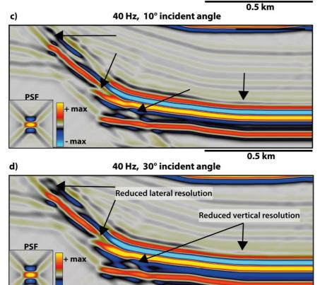
**Figure 5.14:** Effects of varying the angle of incidence on the synthetic seismic of Model 2. a) Represents the geological model, whereas the rest of the images represents the synthetic seismic with different incident angles: b)  $0^{\circ}$ , c)  $10^{\circ}$ , d)  $30^{\circ}$ . The PSF is representing the 2D seismic resolution. Changes in the seismic images are pointed out by black arrows.
