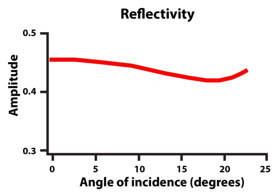
**Figure 5.13:** The effect of an increased angle of incidence on the reflectivity. The reflector represented in this plot corresponds to the boundary between of the low-velocity marls and clays in the overburden (Vp of 2.5 km/s) and the high-velocity limestones below (Vp of 5.5 km/s) in Model 2.
