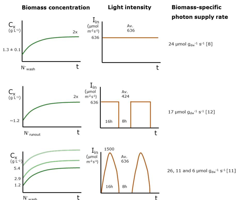
**Figure 1.** Overview experimental conditions used; light regime, average light intensity per day ( $\mu\text{mol m}^{-2} \text{s}^{-1}$ ) and biomass concentration ( $\text{g L}^{-1}$ ) at the onset of nitrogen starvation with their respective average initial biomass-specific photon supply rates ( $\mu\text{mol g}_{\text{dw}}^{-1} \text{s}^{-1}$ ) at the start of nitrogen starvation [8,11,12].
