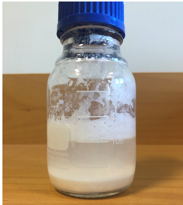
Figure 5.4: Nanofluid collected after 96 hours (before erosion test).
