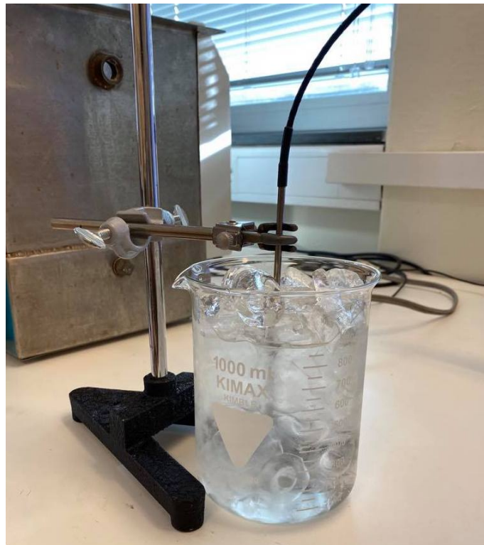
Figure 3.10: Illustration of Pt100 thermometer verification procedure.
