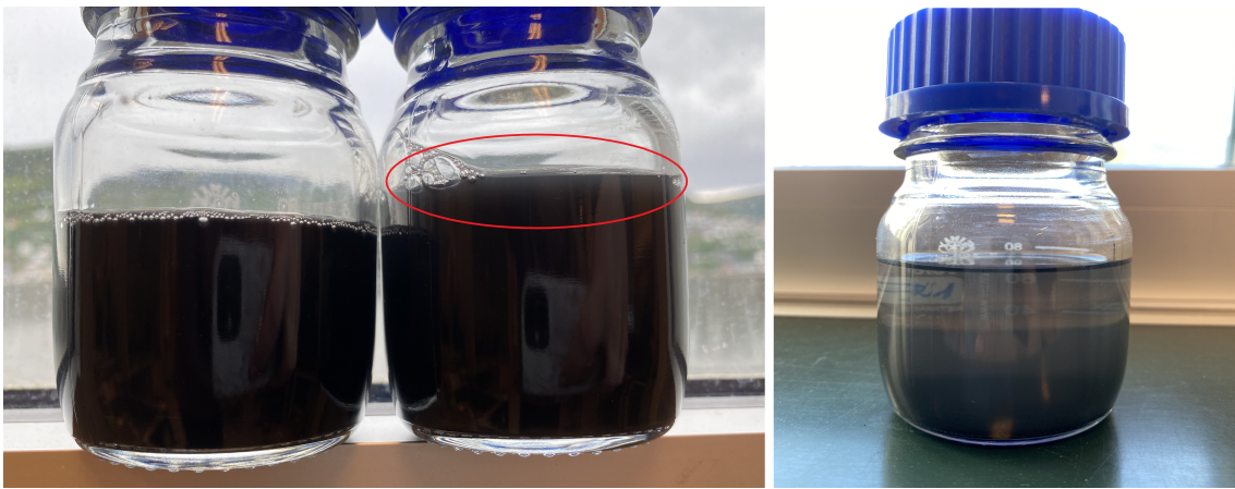
Figure 4.19: Nanofluid samples collected from the reservoir tank. The left photo shows TANK1 after seven days, and TANK2 to the right after collection. The right photo shows sample TANK2 after seven days.
