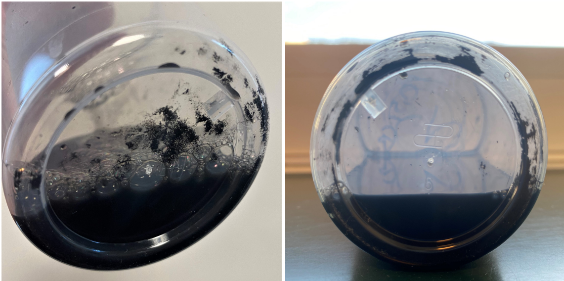
Figure 4.16: Sedimentation on container bottom of reference nanofluid samples after seven days. Sample 1 to the left, and sample 2+3 to the right.
