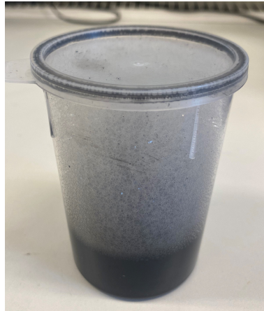
Figure 4.23: Foam generated by shaking a nanofluid sample containing Triton X-100.
