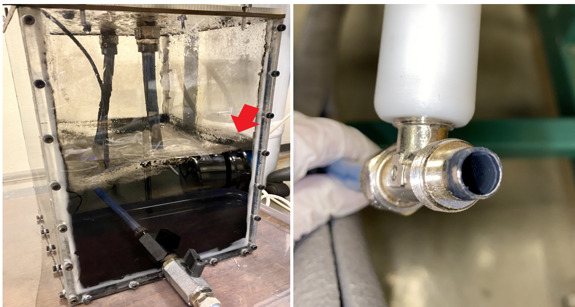
Figure 4.21: Deposition of nanoparticles in the reservoir tank wall to the left, and in a t-pipe joint to the right.
