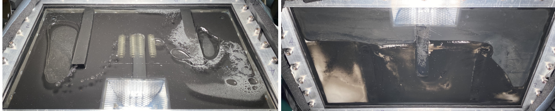
Figure 4.12: Air bubbles inside the DASC under operation. The left photo is of a water DASC experiment with 180^\circ tilt angle. The right photo is of a nanofluid DASC experiment with 45^\circ tilt angle.
