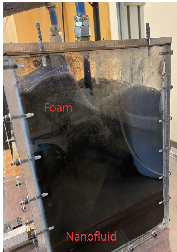
Figure 4.22: Illustration of the foam generation in the reservoir tank.
