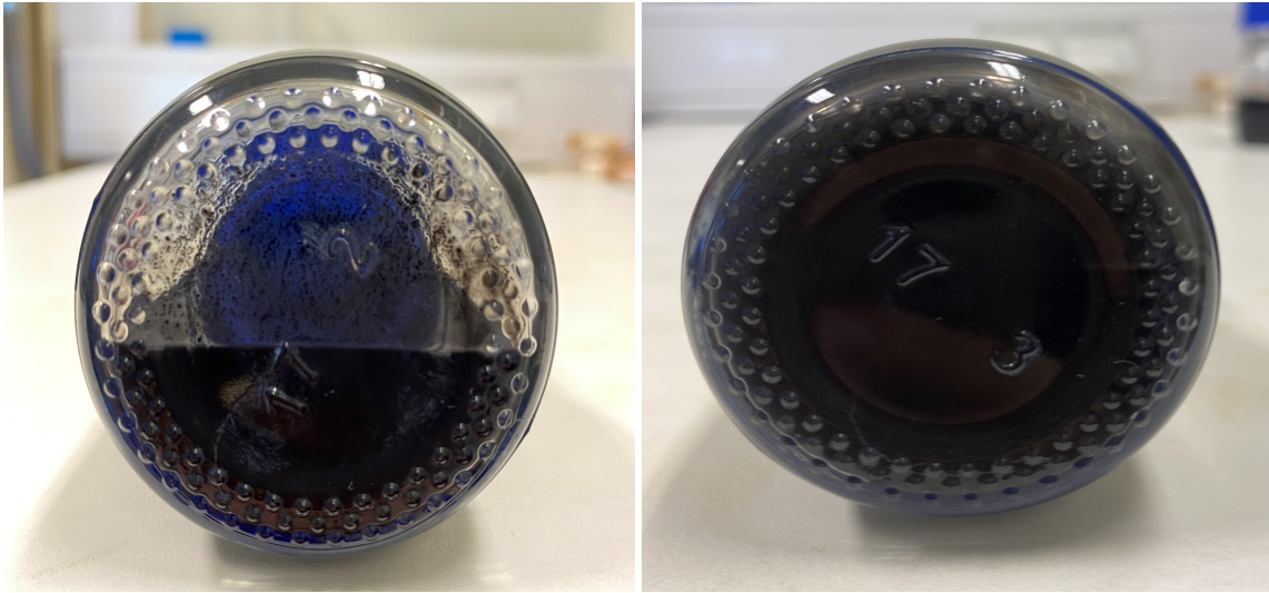
Figure 4.20: Sedimentation in nanofluid samples from the reservoir tank after seven days at rest. Sample TANK1 to the left, and sample TANK2 to the right.
