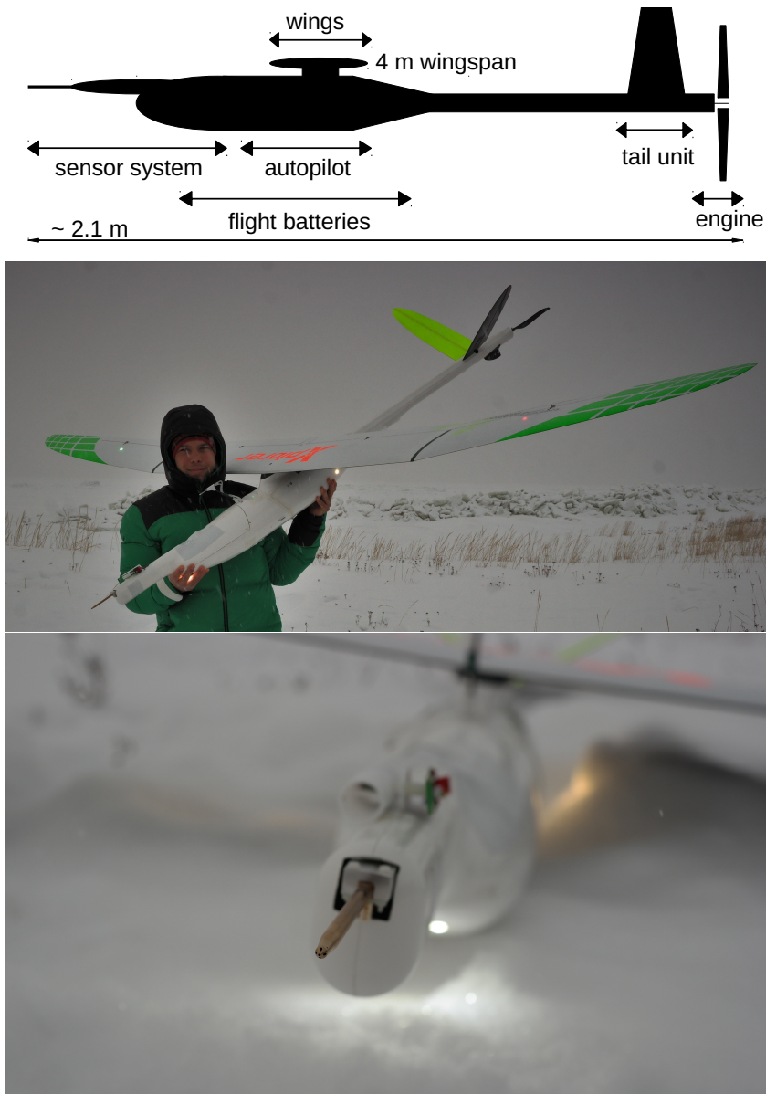
Figure 1. Multi-Purpose Airborne Sensor Carrier (MASC-3) sketch ( top ) and pictures of the airframe with the sensor system ( middle ) and five-hole probe ( bottom ).
