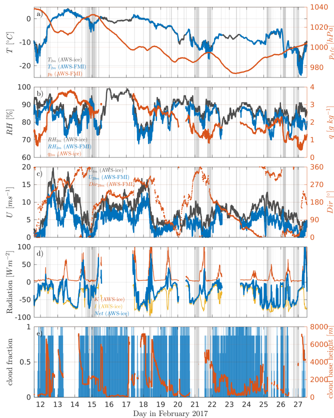
Figure 6. Overview of the meteorological conditions: (a) temperature, T , and surface pressure, p ; (b) relative, RH , and specific humidity, q ; (c) wind speed, U ; and direction, Dir ; (d) short-wave, K , long-wave, I , and net radiation balance, Net ; (e) total cloud fraction and cloud base height. Gray shading indicates times of UAV operation. Note that the wind measurements over land were performed at 29 m above ground.
