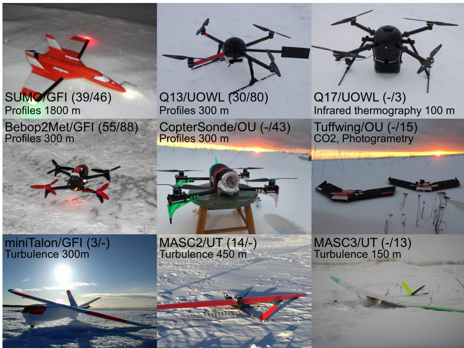
994 FIG. 2. The different UAS systems used during the two campaigns. The numbers of flights are indicated in 995 parentheses for ISOBAR17 and ISOBAR18, respectively.
