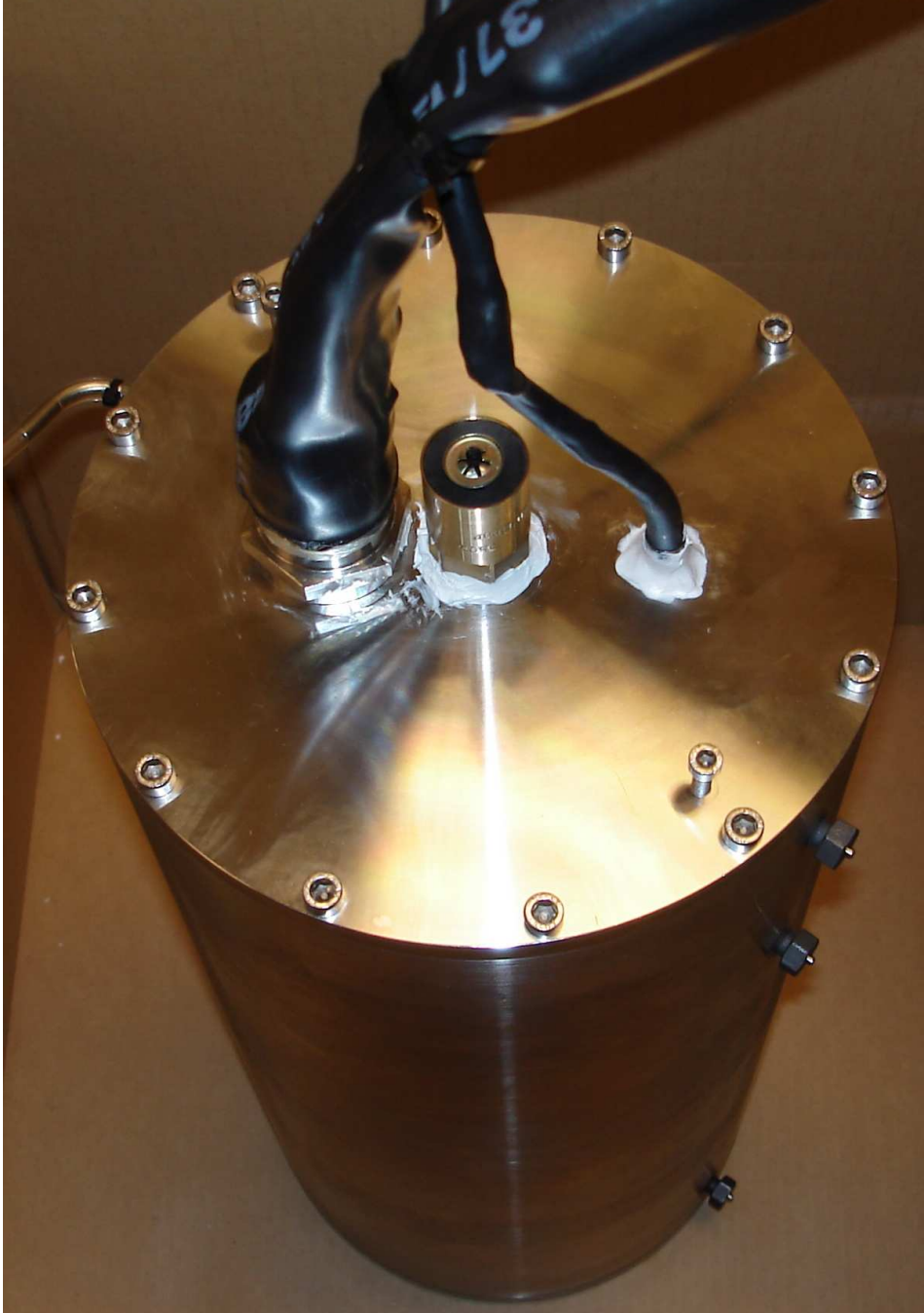
Figure 4.6: Bird view image of the manufactured prototype measurement cell. The three objects at the lid are from left to right cable feed-through connector, safety valve and RH probe.
