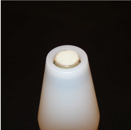
Figure 4.2: The transducer holder developed as part of a doctoral work [93], surrounding the Massa E-188/220 ultrasonic air transducer.
