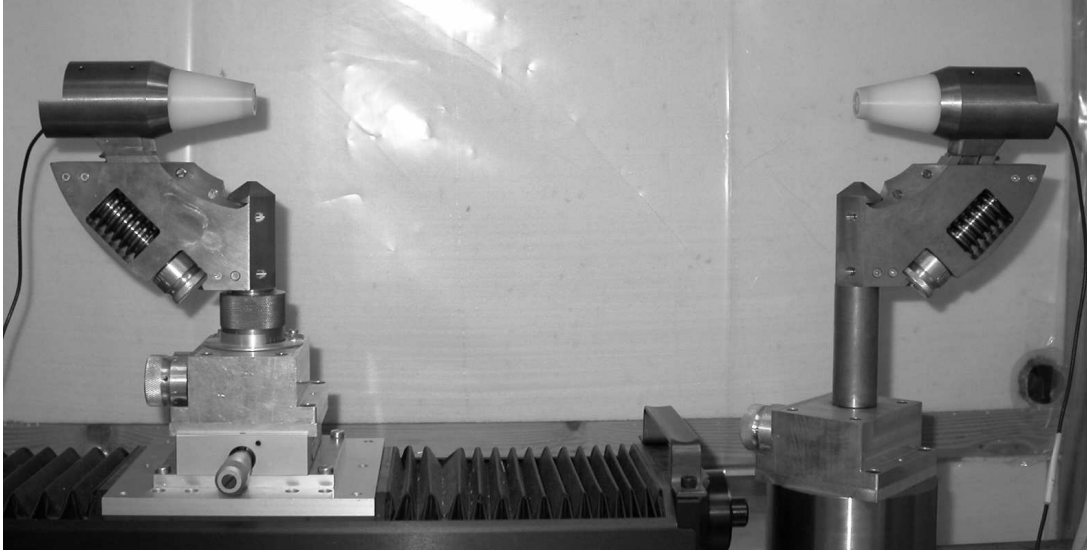
Figure 4.1: The experimental setup of the 2DM. The source and receiver transducer stages are seen to the left and right, respectively. The measurement chamber [PPA] is indicated in the background.
