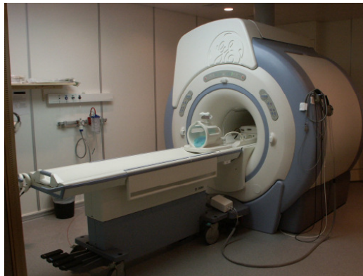
Figure 2: Shown is a Signa series MRI scanner from General Electric, which uses a closed-bore design, in which the person is placed into the middle of the bore.
