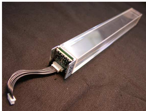
Figure 3.2: A diagram and image of the assembly of a single PHOS cell. The crystal is PbWO_2 . Taken from [16] and [13].
