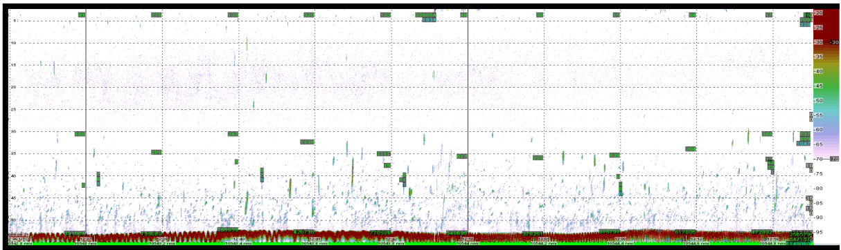
Figure 15 – Echogram from Kerebe Island North. Bottom depth: 51,79 m; horizontal grids seen at every 5 m depth.
