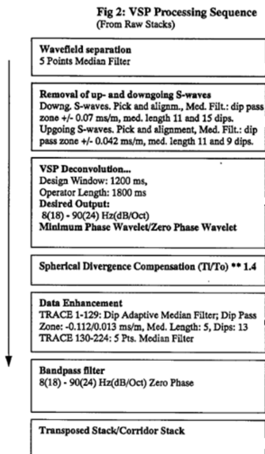
Figure 4-21: Outline of the post-stack processing sequence for NIVSP (Saga Petroleum Report 1993).
