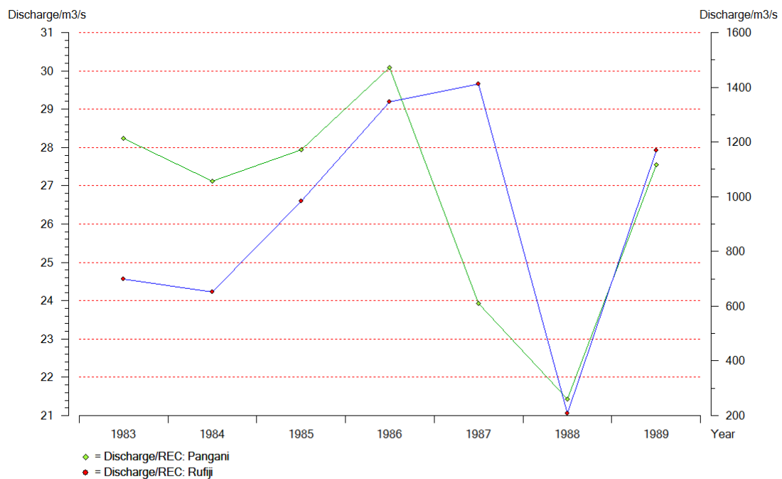
Fig 14: Annual mean discharge of the Pangani river and Rufiji rivers from 1983 to 1989
