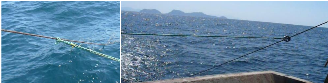
Figure 11: Constrictor rope installed between the warps 100 m ahead of the doors. Left: Constrictor rope affixed to the starboard warp; Right: Purse seine ring attached to the port warp.
