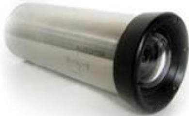
Figure 13: The Navigator monochrome camera used to observe bottom contact of the fishing line and fish behavior in the net mouth area.
