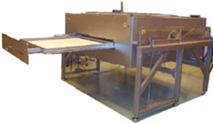
Figure 3.8 The rig can be tilted for horizontal flooding experiments. The shuffle provides easy access to the sample.
