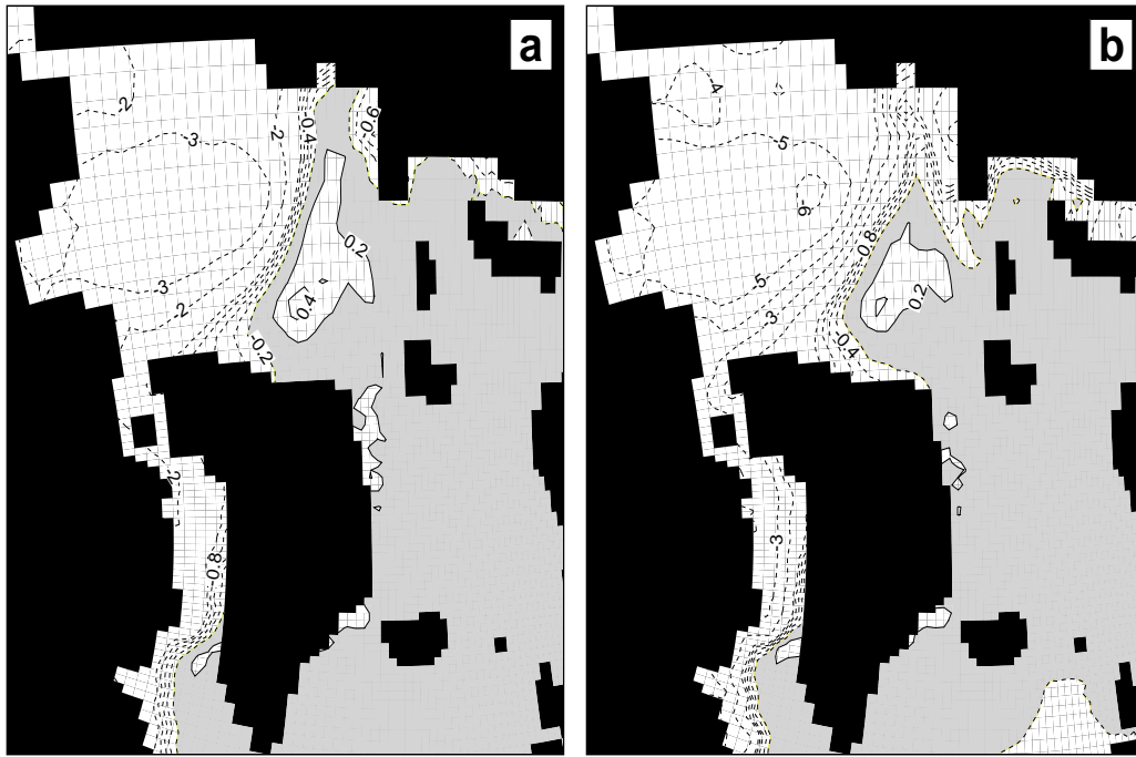
Fig. 11. Difference in the mixed layer density (in \sigma_0 -units) between CTRL and the perturbed simulations. (a) PX2 and (b) PX5. Contour interval is 0.2 between -1 and 1 , and 1 elsewhere. Negative values indicate reduced density.
