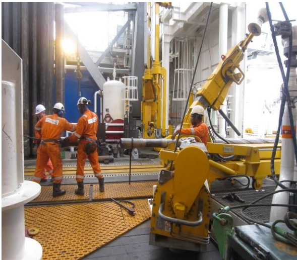
Plate 11: Ghanaian roughnecks connecting pipes on a rig.
