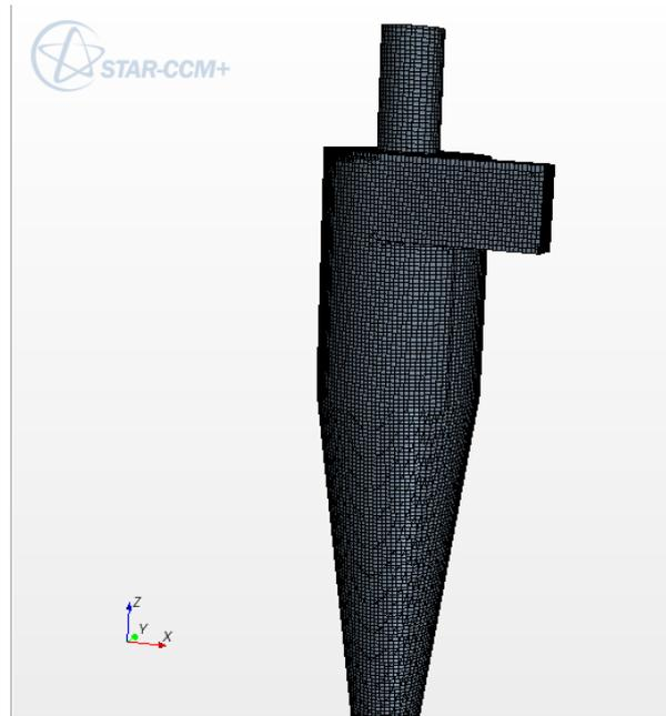
**Figure 2.17:** Mesh applied over the domain of interest, called a volume mesh
