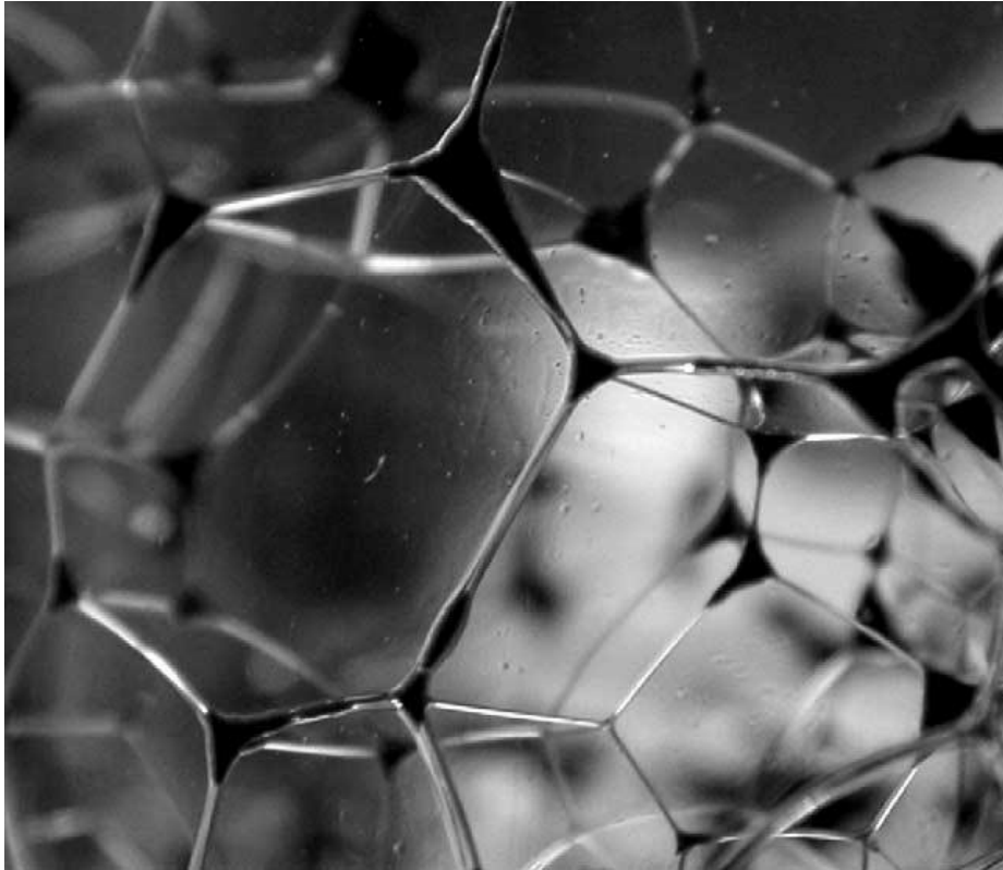
Figure 2-8 – A picture showing foam with a plateau border with an oil film. The picture is taken 24 hours after mixing and is enlarged four times. (Vikingstad et al., 2005)
