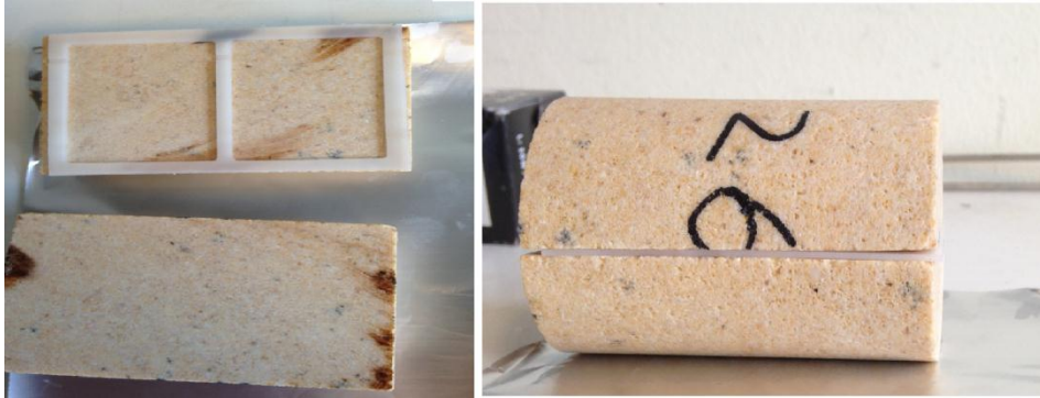
Figure 3-7 – picture to the left showing open core with spacer and picture to the right showing a closed core with spacer in the middle
