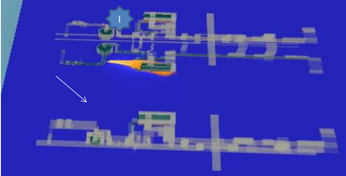
Figure 9 Scenario 2; Jet fire after 60 seconds.
