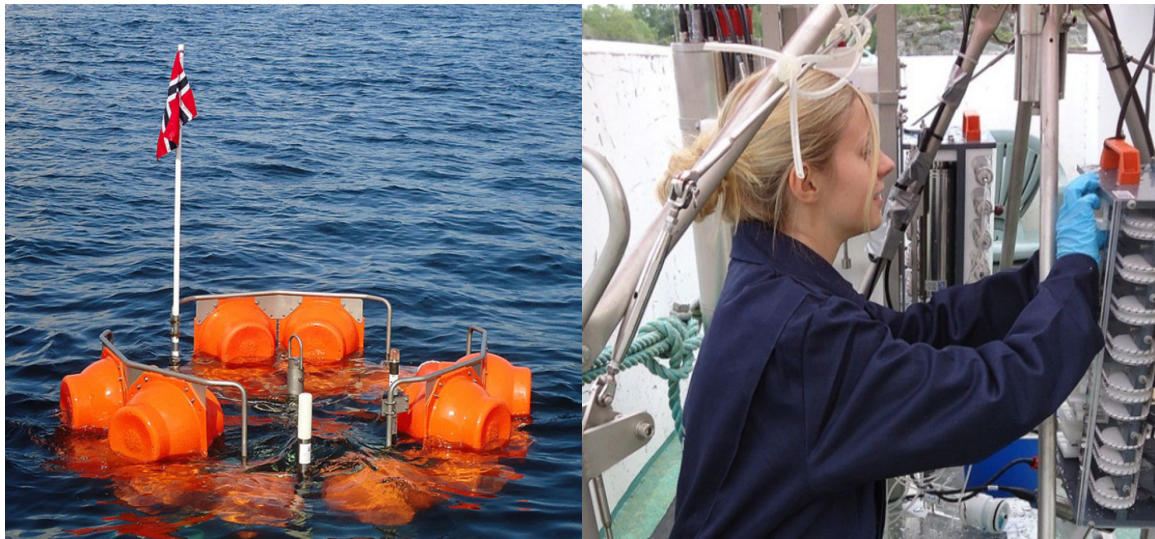
Figure 2: The Aquarius lander used in this in situ mimick of a CO 2 leakage.. A) The Aquarius lander floating in he water after recovery from the seafloor. B) Handling water sample syringes on one of the two lander chambers after lander is back on ship deck.
