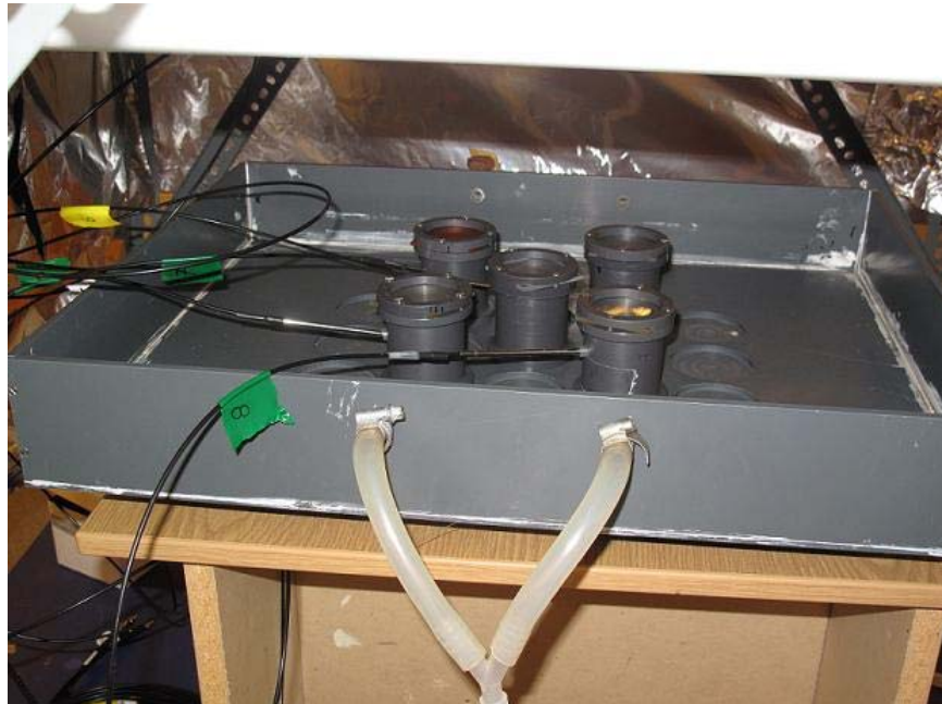
Figure 4.5: The set up of the water bath with the sample bottles in the photoinhibitor.
