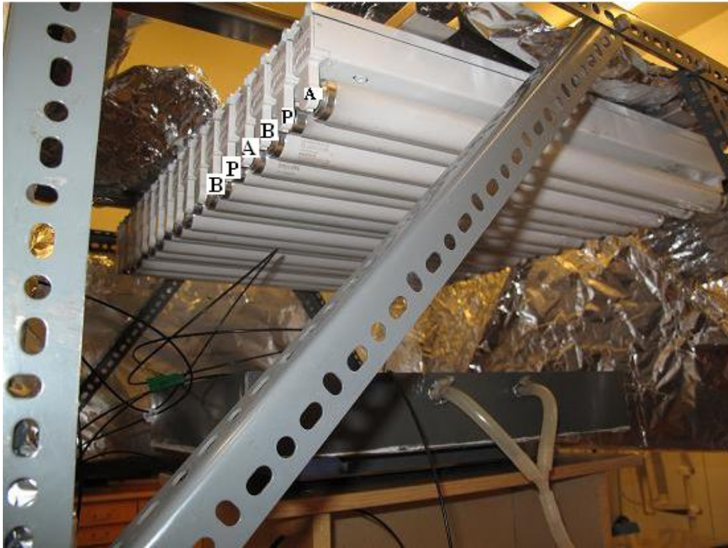
Figure 4.1: The arrangement of the florescent lamps in the photoinhibitor. P-represents PAR, A-UVA and B-UVB.
