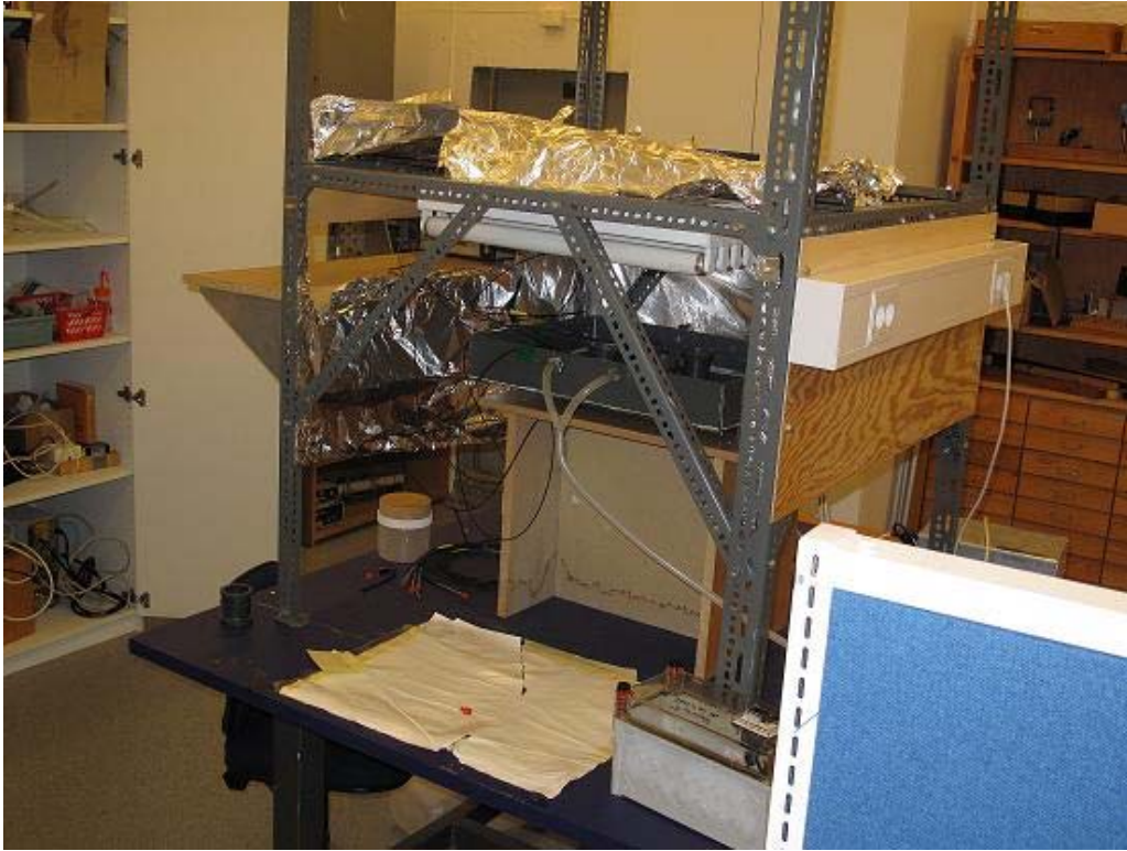
Figure 4.4: The complete set up of the photoinhibitor used to expose algae to different wavelength of light.
