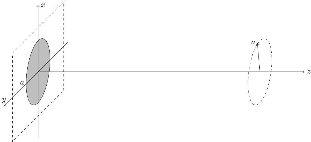
Figure 2.2: Sketch of a piston source model, where the piston has radius a . A circular acoustically transparent circular receiver, also with radius a , is placed coaxially to the source at a distance z .
