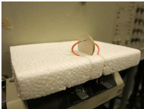
Figure 3.4: A polystyrene holder is used when measuring the admittance of single piezoelectric ceramic disks, with the disk placed loosely in a wide groove in the polystyrene.
