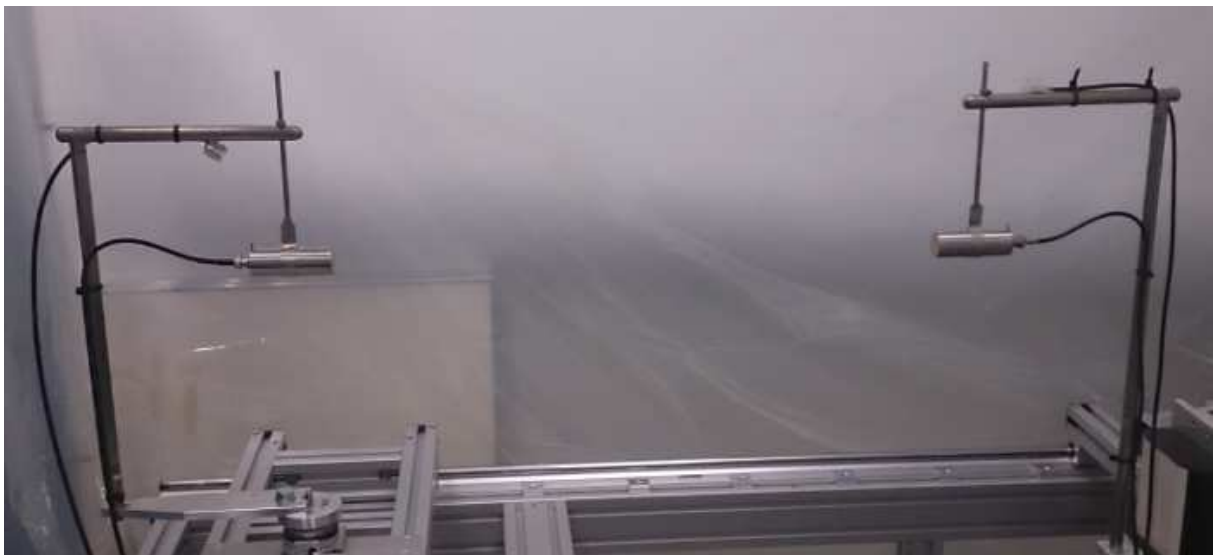
Figure 3.14: Two piezoelectric transducers developed during the present work with a separation distance of 66 cm.
