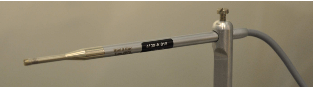
Figure 3.12: A Brüel & Kjær 4138-A-015 microphone system mounted on an aluminium rod.
