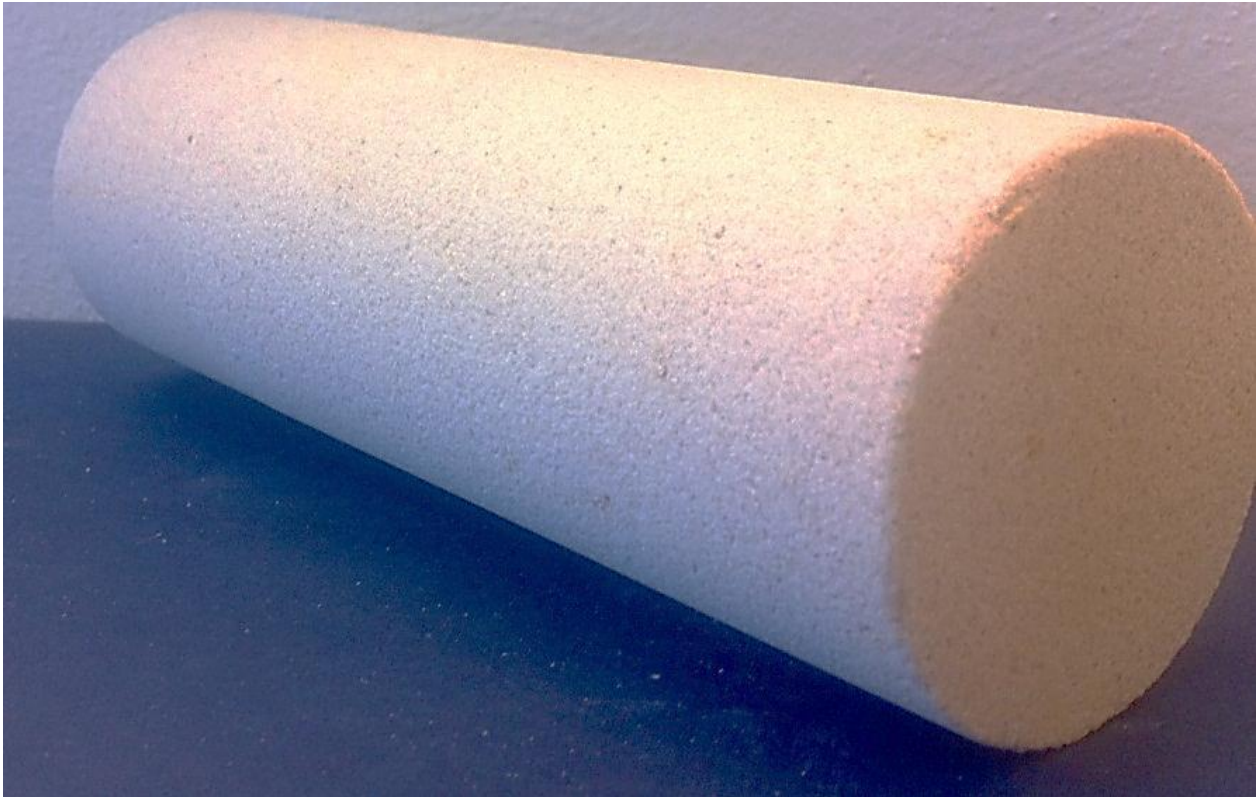
Figure 2-3: Picture of a Bentheim sandstone core used in one of the experiments conducted during this thesis. The core was approximately 14 cm long and 5 cm in diameter.
