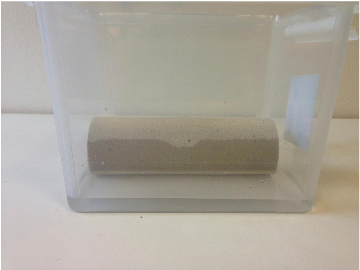
Figure 2-6: Picture of a spontaneous imbibition when saturating a water-wet Bentheim sandstone core. The brine is only covering the bottom of the tray, but due to wettability and capillary pressure the water will imbibe and distribute itself in the porous media.
