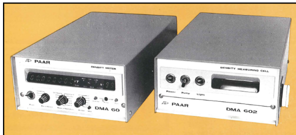
Figure 2.1: DMA 60 processing unit (left) and DMA 602 measuring cell (right) [56]. The in- and outlet where sample is introduced and discharged is shown on the right hand side of the measuring cell. A constant temperature circulator is connected to the measuring cell (not shown), providing continuous flow of thermostatted water surrounding the u-tube.
