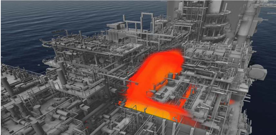
Figure 3-4 Flowvis plot. A representation of an ignited gas release in an offshore installation, [23].
