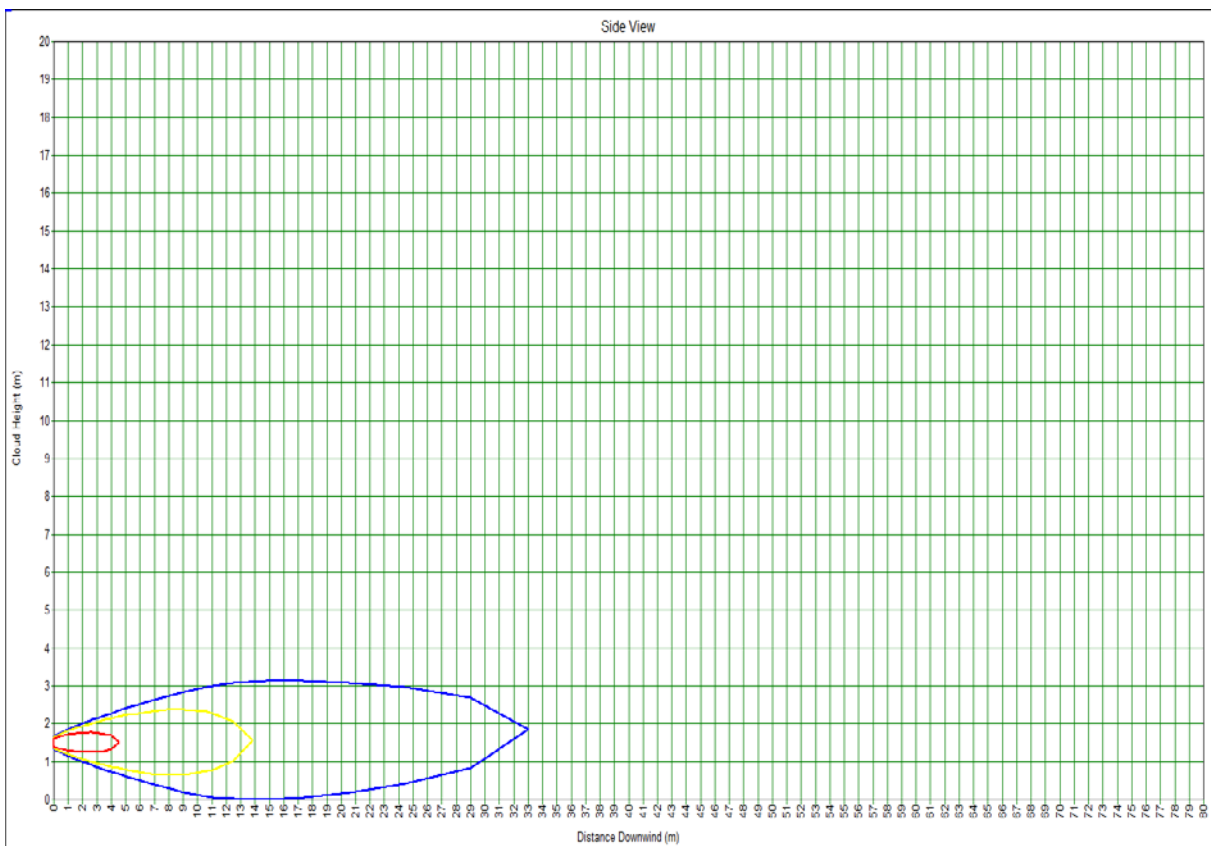
Figure 5-11 Side view plot; PHAST method2 10.0D jet release of medium sized release (3.93 kg/s). (The UFL value is shown by the red color, yellow represents the LFL concentration extent and blue represent LFL 2 . FLACS comparison plot is 260306 shown in Figure 5-9.
