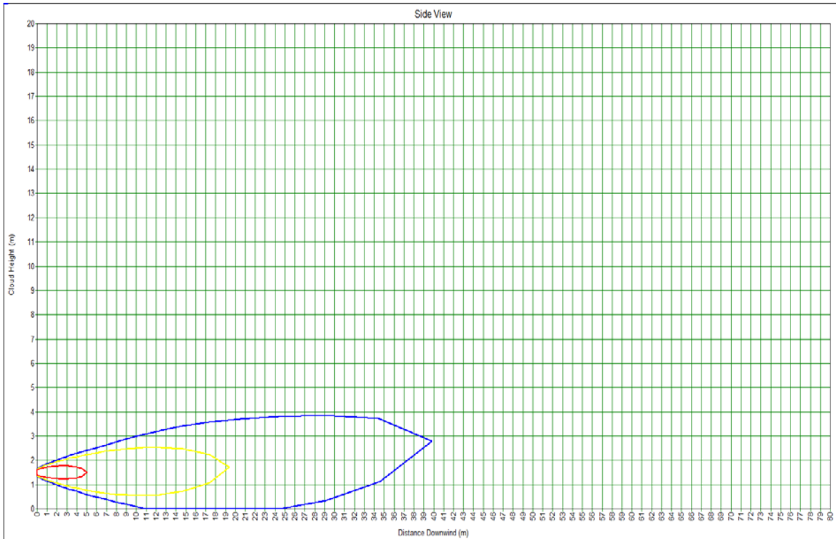
Figure 5-10 PHAST method2 jet release of medium sized (3.93 kg/s) of wind conditions of 3.0 m/s stability B. (UFL is indicated by the red color, yellow represents the LFL concentration extent, and blue represent the LFL 2 range. FLACS comparison plot is 260303 shown in Figure 5-9.
