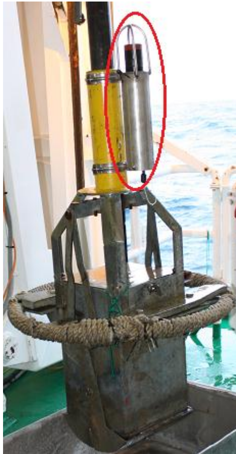
Figure 2.5. The box-corer and the transponder (marked with a red circle). Photo: Janita Flo.
