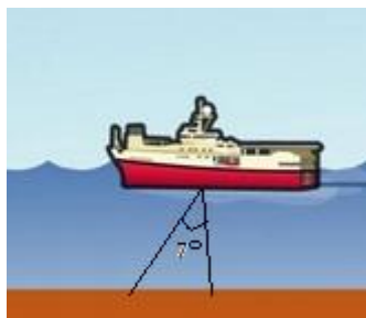
Figure 2.1. Illustration of the detection radius of Simrad EK60 system.
