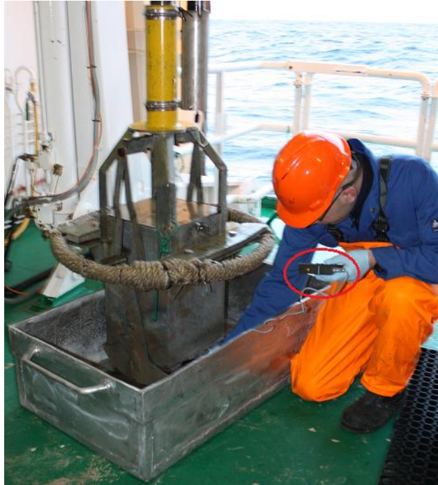
Figure 2.6. The radiation level was checked with an Automess dose rate meter (marked with a red circle). Photo: Janita Flo.
