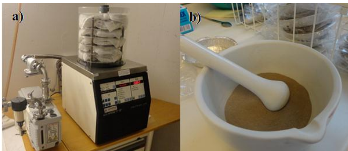
Figure 2.9. (a) Samples getting freeze-dried in the CHRIST ALPHA 1-4 freeze dryer with Edwards RW3 vacuum pump, and (b) a sample getting homogenized using a mortar.
