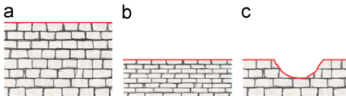
Figure 3.3: (a) Texture on the initial configuration of a layer; (b) compacted layer which is communicated by a compacted texture; (c) eroded layer which is communicated by a cut texture, where no texture deformation is performed. Image courtesy of Endre Lidal [73].
