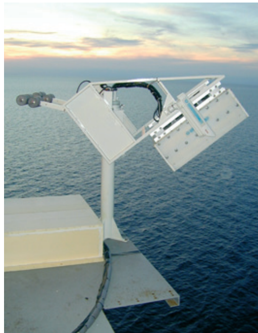
Figure 5a. LAURA during its installation on the Casablanca oil rig, 32 m above the sea surface, and during measurement taking on a calm day
