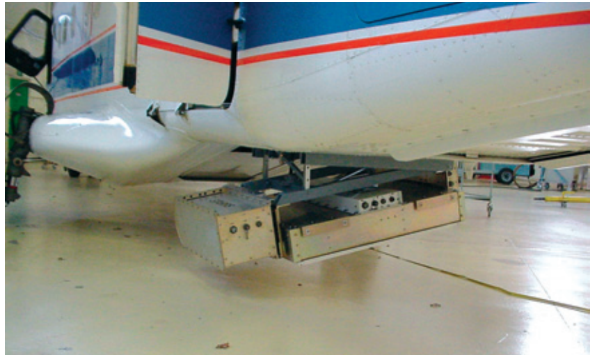
Figure 9. STARRS mounted on the DO228 aircraft in data-acquisition configuration (tilted). For take-off and landing, the instrument was moved into a horizontal position using a winding device specially designed for this campaign
