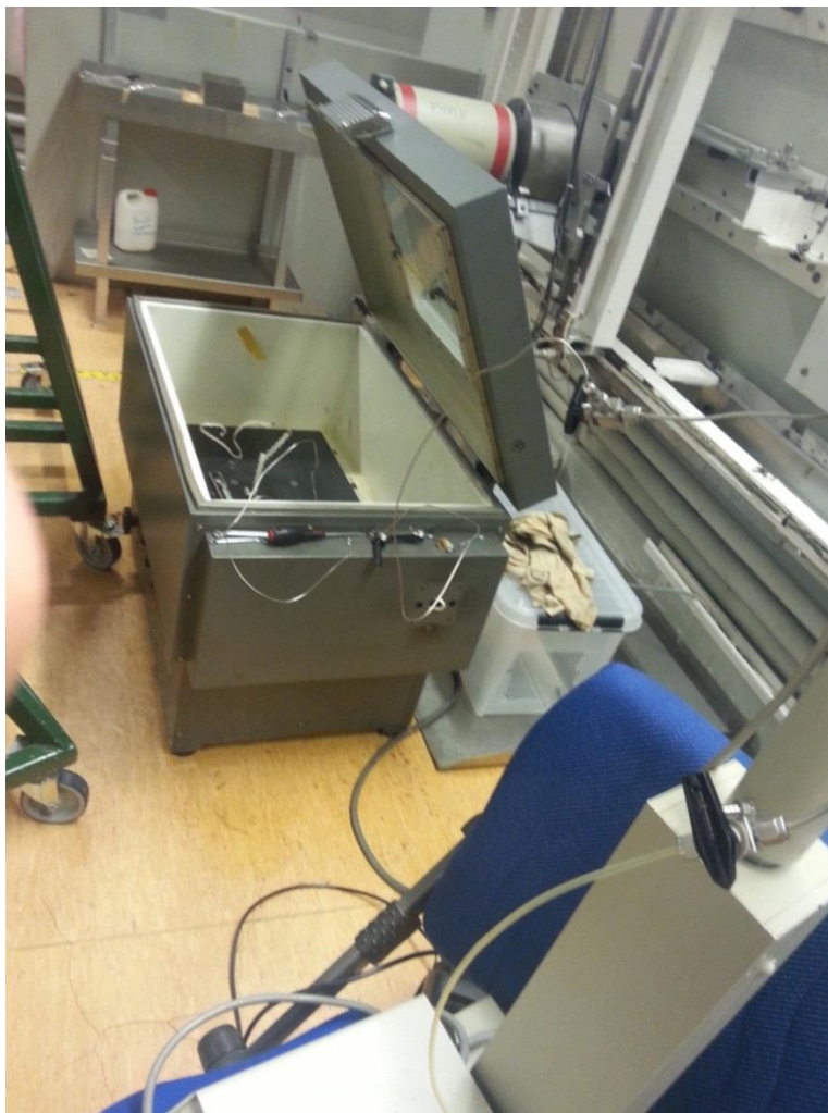
Figure 4-2. The shaker used for mixing of the live brine. The buffer was strapped to the bottom of the shaker, which was set for desired temperature, and connected to the ISCO pump in the front of the picture set to keep constant pressure.
