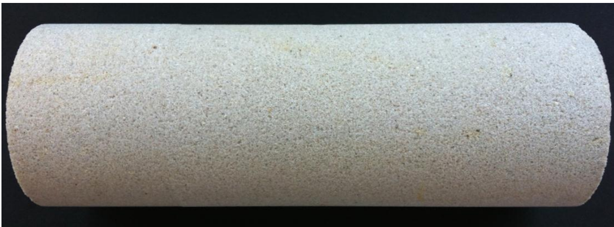
Figure 4-1. Bentheim sandstone core. The diameter is around 5cm and the length is around 14cm.
