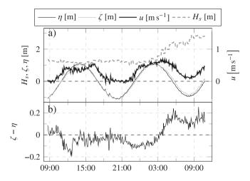
**Fig. 6.** a): Measured current speed, sea surface heights and significant wave height from October 30-31, 2012.  $\eta$  and  $H_5$  are measured by the outer RBR (cf. Fig. 1),  $\zeta$  and u are measured inside the lagoon, by the inner RBR and SeaGuard, respectively. Note the different scale for u. b): Measured sea level difference between the inside and the outside of the lagoon.
