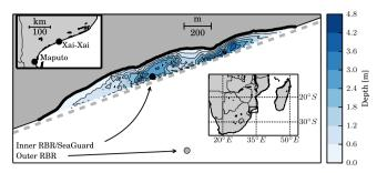
**Fig. 1.** Map showing a GPS track along the shoreline (thick black line) from October 2013, and bathymetry measured by echo sounder in October 2011. Instrument positions from survey in October 2012 are indicated. The dashed grey line indicates the approximate position of the reef. The insets show the location of Xai-Xai in southern Africa.
