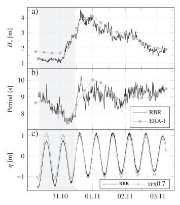
**Fig. 2.** Comparison of measurements by RBR with ERA-Interim and the TPXO.7 tidal model for October—November 2012. a) shows significant wave height (ERA-I), b) shows mean wave period (ERA-I) and c) shows tidal elevation (TPX). The grey shading indicates the period when concurrent measurements were made inside the lagoon, i.e. that displayed in Fig. 6.
