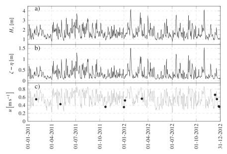
**Fig. 9.** Daily maxima of a) significant wave height ( $H_s$ ) from ERA-Interim; b) modelled  $\zeta - \eta$  and c) modelled u, from a two year long simulation where modelled data from ERA-Interim and TPXO.7 was used to force the model. The black dots indicate dates where accidents have been reported at Xai-Xai.
