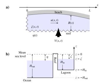
**Fig. 3.** Schematic view of the system. Panel a) shows variations in *x*, while panel b) shows a cross section of reef, indicating different depths for a situation near low tide.
