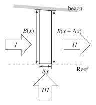
**Fig. 4.** Schematic illustration of the terms in continuity equation. The schematic shows a control volume in the lagoon. The change in volume is determined by what flows into it from the left (*I*), what flows out on the right (*II*) and what comes across the reef (*III*).
