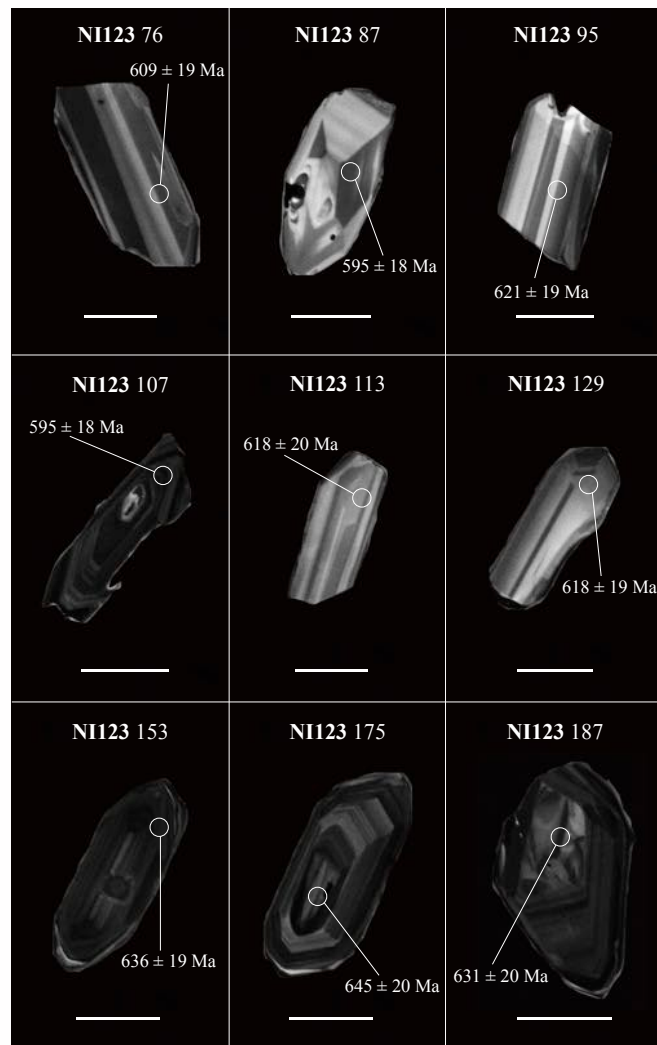
Fig. 31: Cathodoluminescence images of characteristic zircons in NI123 migmatitic gneiss. The circles show the laser ablation points on the zircons, and the scale bars show 100 \mu\text{m} .
