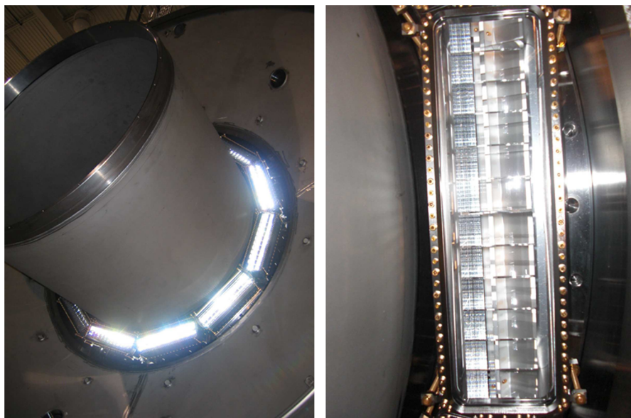
Fig. 59. DIRC SOB: Inner cylinder and the windows of several of the 12 bar boxes (left), and the face of a bar box showing the ends of 12 fused-silica bars (right).
