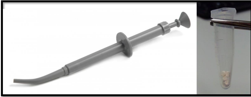
Figure 20. Amalgam carrier provided standard volume of material plugs (Left). Four material plugs were used for creating stock material eluate solution (Right).
